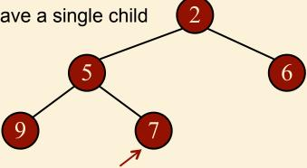
☐ The last node of a heap is the rightmost node of depth *h*
